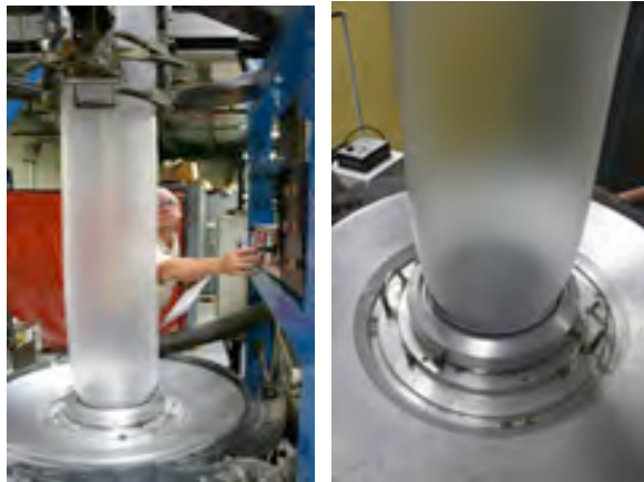
Vice president of manufacturing & technology David Collette examines the film bubble on Argotec's blown film laboratory extrusion line.
