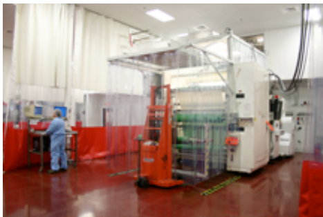
Argotec's seven cast-on-carrier and flat-die extrusion lines are housed in an 8,000 square-foot hard wall clean room and enclosed in their own Class-10,000 soft wall clean room to ensure extremely clean ArgoThane™ polyurethane film & sheet.
