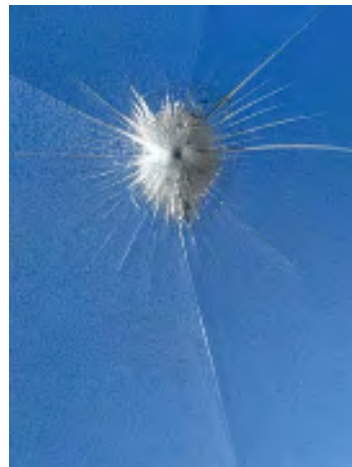
Fig. 11 Super-strong glass composites made with Argotec optical interlayer films are used in armored vehicles, correctional facilities, banks, and other commercial and military applications where ballistic glass is needed
