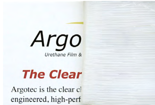
Fig. 3 Polycarbonate sample buckles, cracks and fogs to an opaque white (right half of photo) when MEK solvent penetrates TPU-TPU edge seal material wrapping.
