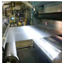
Argotec's camera inspection system helps ensure customers receive super-clean optical interlayer films
