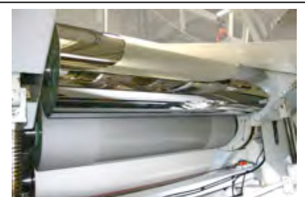
Aliphatic optical interlayer film being extruded in hard-walled cleanroom at Argotec's Adams Road optical films facility
