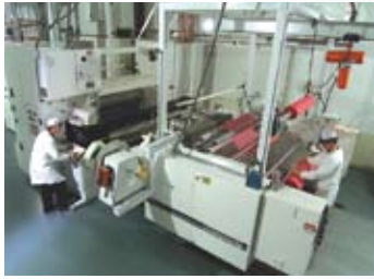
Flat-die extrusion in Argotec's hard-wall cleanroom production facility
