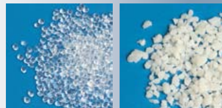
Virgin TPU resin (left) and regrind
